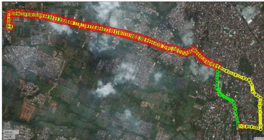
Figure 9. The coordinates of path C (green color) and path D (yellow color) after interpolation, the equivalent coordinate points (red color)
