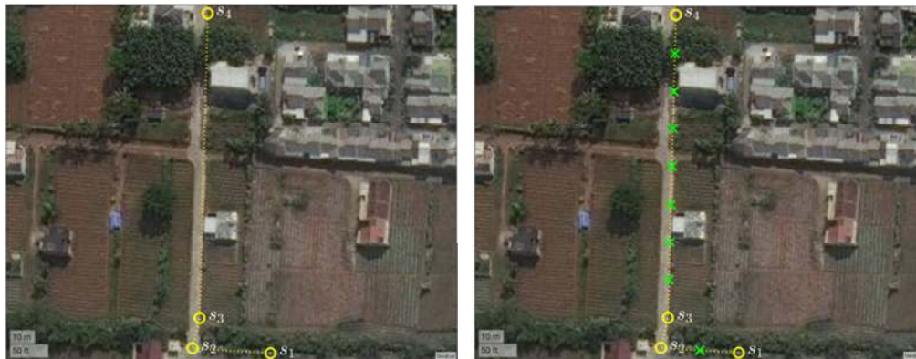
Figure 3. Coordinate points in path s before (left) and after adding interpolation points (right).
