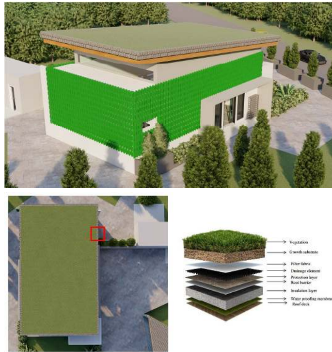
Figure 7. Green roof applied on the mosque
