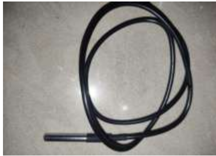
Gambar 8. Sensor suhu DS18B20
