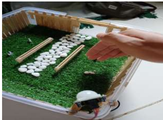
Figure 5. The condition of the Door Cage is Open and the PIR Sensor Detects Movement
