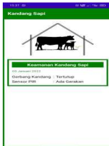
Figure 4. Smartphone Display When the PIR Sensor Detects Movement but the Door is Still Closed
