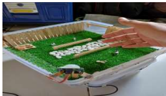
Figure 3. PIR Sensor Detects Motion but Door is Closed
