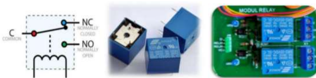
Figure 2. Symbols and Forms for DC Relays
